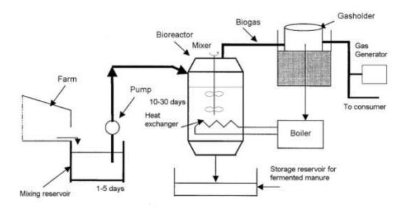
Fig. 7.4. The technological scheme of biogas production
