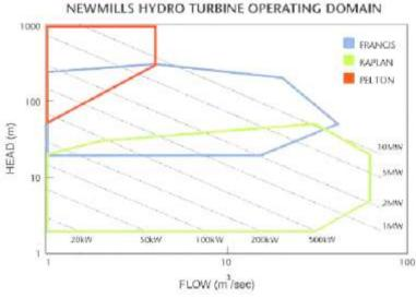
• Fig. 10.3. Typical operating ranges (water discharge and head) for different types of turbines: Kaplan and propeller turbines, Francis turbines, and Pelton turbines manufactured by Newmills Corporation
