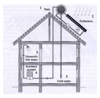
Fig. 3.2. Solar water heating system with thermosiphon circulation: 1-tank, 2-collector, 3 –hot water, 4 – auxiliary system, 5-cold water
