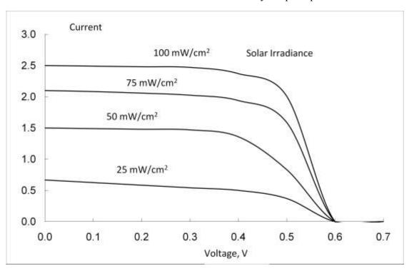
Fig. A.1. Current-Voltage curves (I-V curves) for solar photovoltaic cell at different values of solar irradiation (in mW/cm²)
