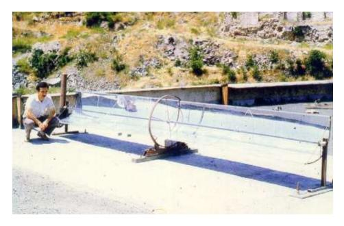
Solar Parabolic Trough Collector installed at the roof of SEUA
