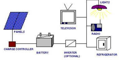
Fig. 5.4. Stand-alone (off-grid) PV system
