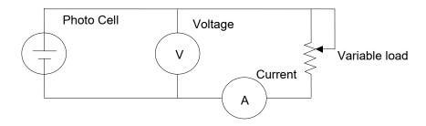
Fig. A.2. The electrical scheme of measurements of voltage and current of solar photovoltaic cell.
