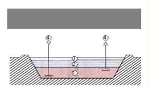
Fig. 4.5. Solar pond: 1 – water layer with high concentration of salt, 2 – water layer with intermediate concentration of salt, 3 – water layer with low concentration of salt, 4 – input of cold water and discharge of warm water.
