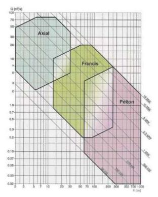
Figure 10.4. Turbines' type field of application [52]
