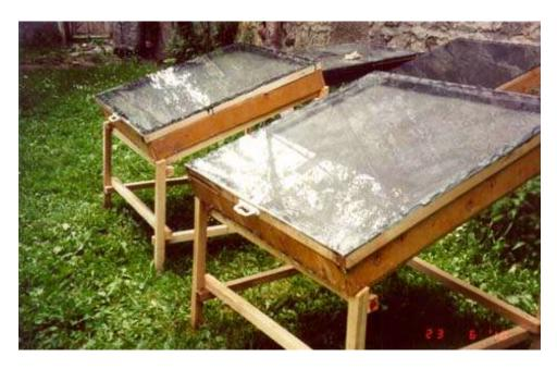
Solar dryers developed in Vanadzor (2010)
