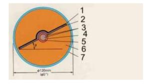
Fig. 3.6. Cross section of evacuated tube [1] 1 – selective coating, 2 – absorbing plate, 3 – heat-transfer fluid, 4 – outer surface of copper pipe, 5 – inner surface of copper pipe, 6 – evacuated space, 7 – glass tube (width of walls is 2mm), diameter of glass tube is126mm (5 inches)
