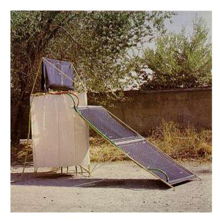
Bathroom operated through solar water heating
