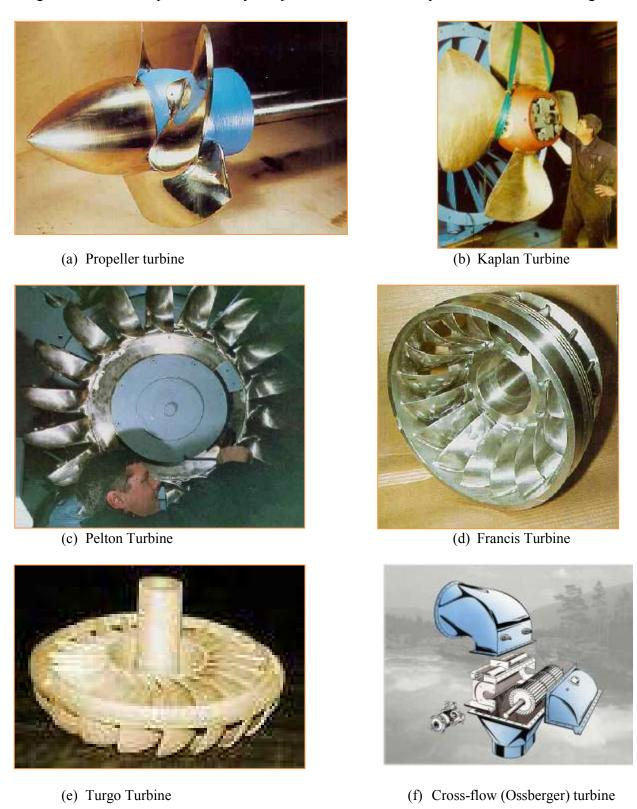
Fig. 10.2. Different types of hydraulic turbines: a - Propeller turbine, b - Kaplan Turbine, c- Pelton Turbine, d- Francis Turbine, e- Turgo Turbine, f- Cross-flow (Ossberger) turbine.
