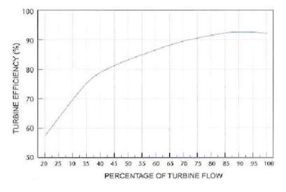
Fig. 10.5. Francis type turbine efficiency curve
