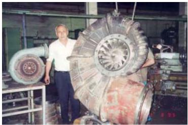
Fig. 10.9. Frencis type turbine manufactured in Armenia by Vorotan LLC
