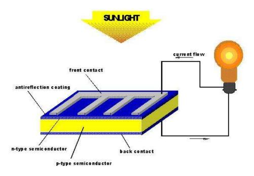
Fig. 5.1. The structure of PV-cell: 1 – anti-reflection coating, 2 – front electrode, 3 - n-type silicon, 4 - p-type silicon, 5 – back electrode, 6 - current, 7 - sunlight
