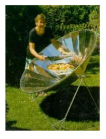
Fig. 3.7b. Parabolic dish solar cooker
