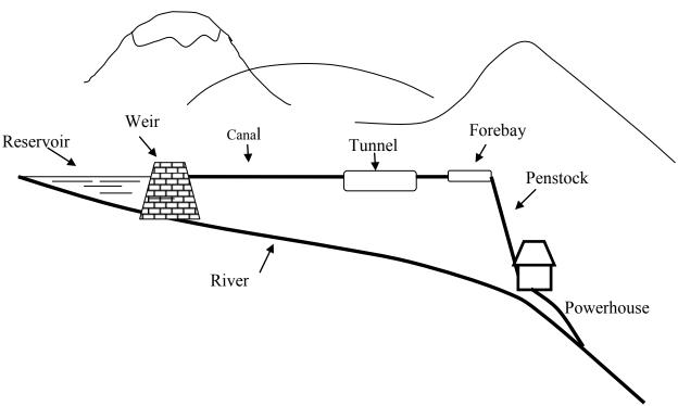
Fig. 10.1. Typical layout of small HPP
