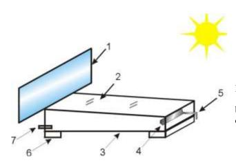
Fig. 3.8. Solar distillation unit: 1 – reflective surface, 2 – glass cover, 3 – collector with black bottom, 4 – fresh water trough, 5 – fresh water drain pipe, 6 - support, 7 – inlet pipe for polluted water
