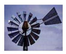
Fig. 8.5. Low-speed (multi-blade) WPP
