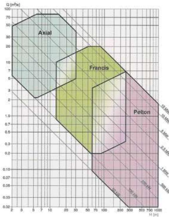
Figure 10.4. Turbines' type field of application [52]
