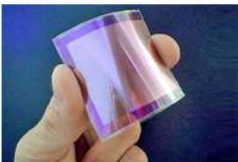
Fig. 5.6. Thin film PV cells manufactured by Nanosolar company
