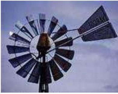
Fig. 8.5. Low-speed (multi-blade) WPP
