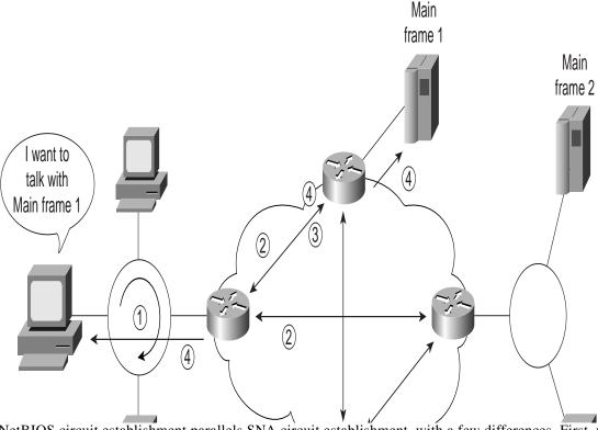
Figure 29-6 DLSw Circuit Establishment Flow
