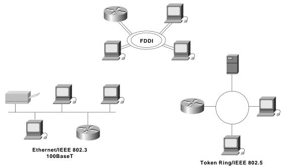
Figure 2-1 Three LAN Implementations Are Used Most Commonly
