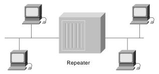
A *hub* is a physical layer device that connects multiple user stations, each via a dedicated cable. Electrical interconnections are established inside the hub. Hubs are used to create a physical star network while maintaining the logical bus or ring configuration of the LAN. In some respects, a hub functions as a multiport repeater.
