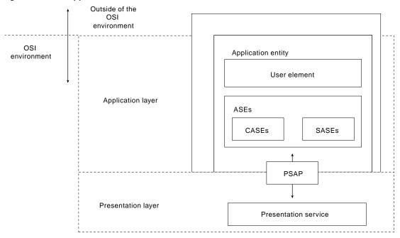
Figure 30-5 An Application Process Relies on the PSAP and Presentation Service
